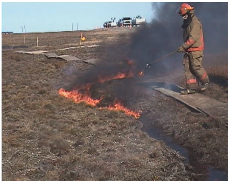
Igniting Oiled Tundra from a Plywood Platform
