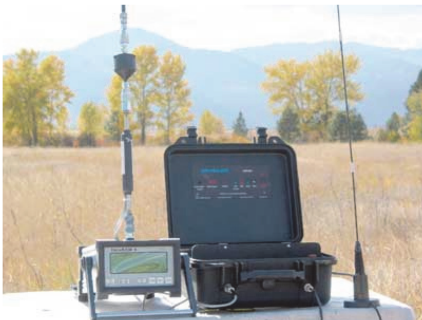
Example of a Field-Deployable Particulate Monitor that Uses Light Scattering Technology
