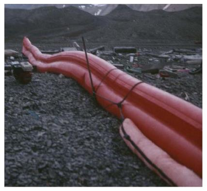
Water-ballasted ("shore-seal") boom placed across the intertidal zone of a beach to prevent oil moving along shore. A length of sorbent boom (pink colored "sock boom") is attached to the lower (intertidal) portion of the shore-seal boom (field trials on oiled beaches, Svalbard).
