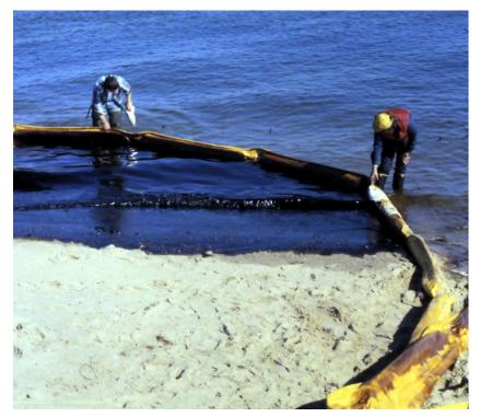
Conventional floating boom with skirt buried in the intertidal beach sediments to collect oil moving along shore (field trials, New Jersey).
