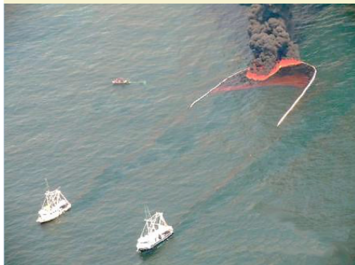
FIGURE 1. ISB conducted on the water by containment within a fire boom. (Mabile 2012)
