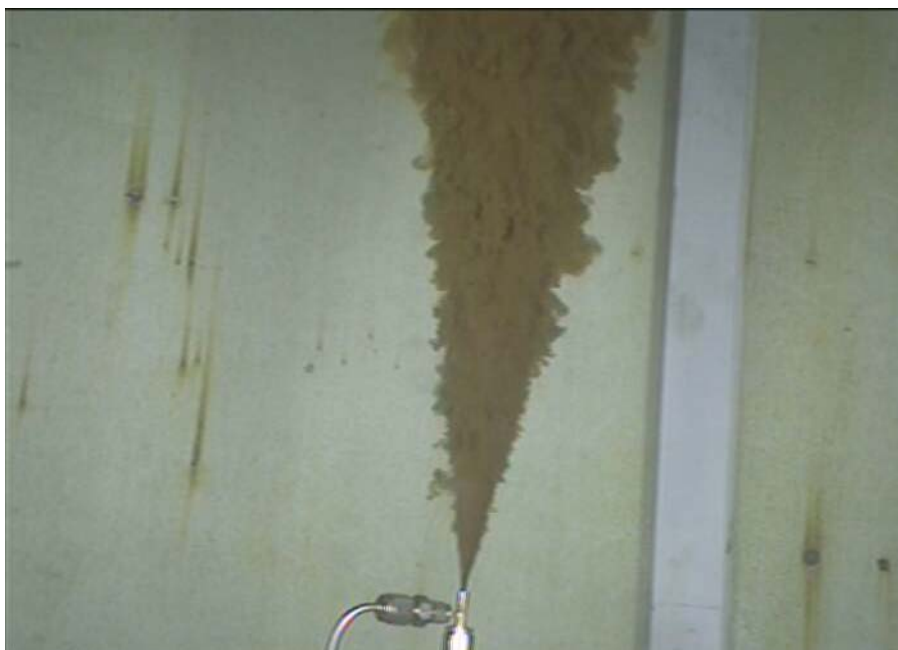
Figure A - 3: Screen Capture of Video during High Pressure Test, Dispersant Introduced (1% C9500)
