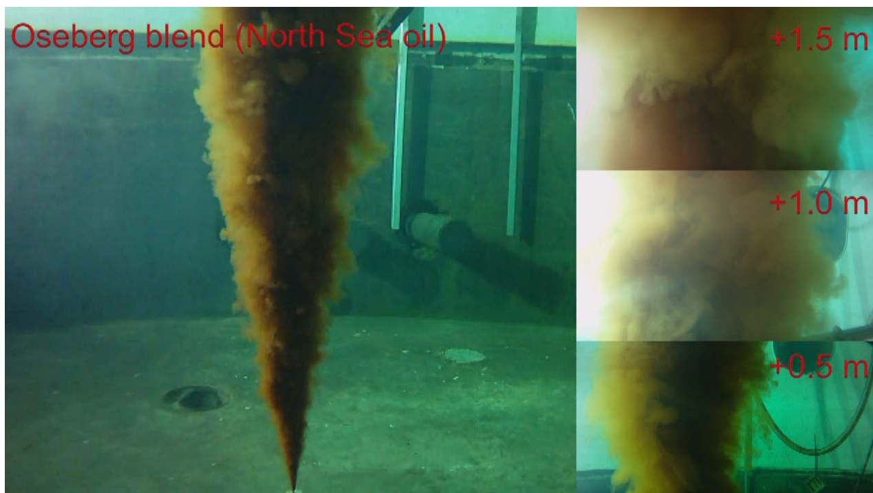
Figure A.8.7: An example of a composite video showing the four HD cameras covering the rising oil flume at 0.5 m intervals over the release point. This is from earlier experiments with a North Sea crude (Oseberg blend).
