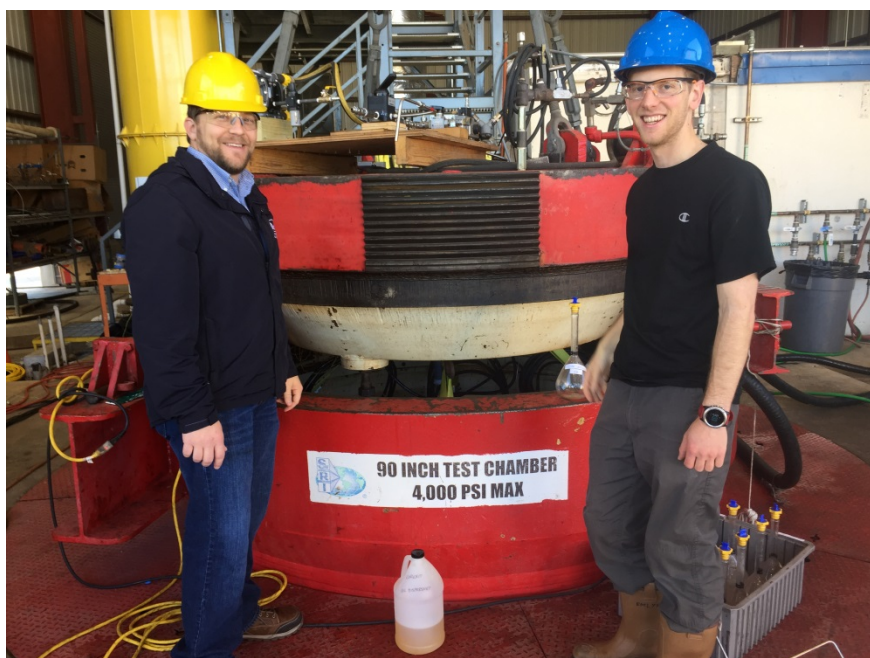
The 90" hyperbaric chamber at SwRI before the lid is lowered and closed
