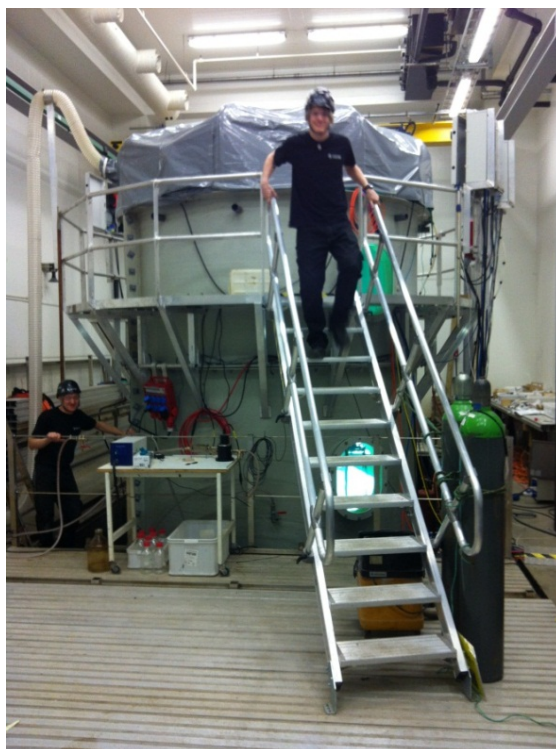
Figure A.3: The Tower Basin per March 2012 showing the scaffolding, staircase and the railings to ensure safe working conditions and the ventilated hood.
