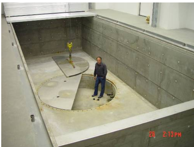
Figure A.1: Ice basin without propellers and other equipment used for circulation showing the fundament for the Tower Basin (left) and the initial mounting of the Tower Basin in January 2011 (right).
