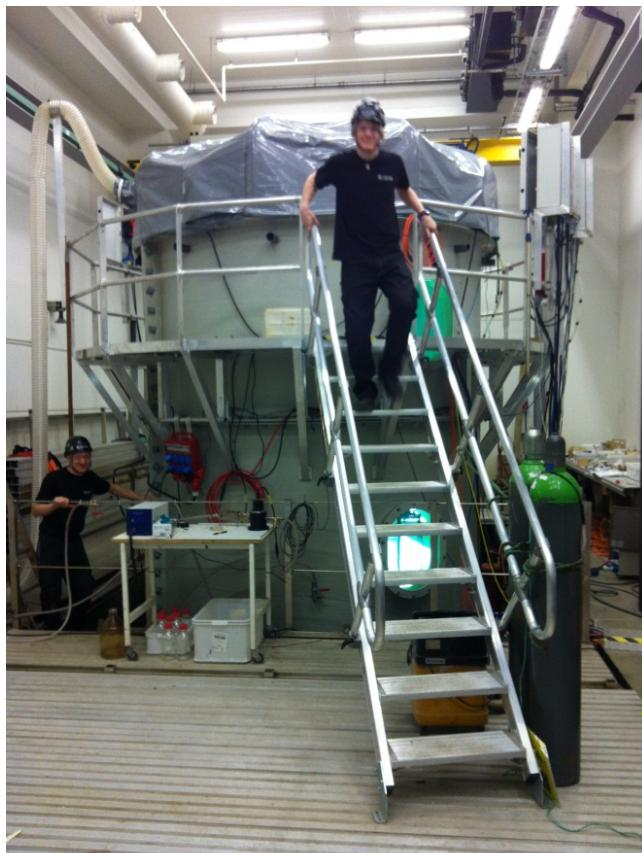
Figure 4.4: The Tower basin per March 2012 showing the ventilated hood, scaffolding, staircase and railings to ensure safe working conditions.
