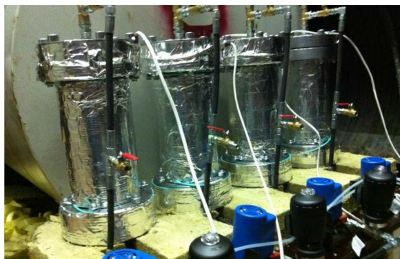
Figure 4.2: The new system with four 7 L tanks to heat the oil. Heating coils were wrapped around the tanks and covered with aluminium foil. The tanks were also insulated with foam (removed for this picture). The blue objects are pumps for internal circulation.
