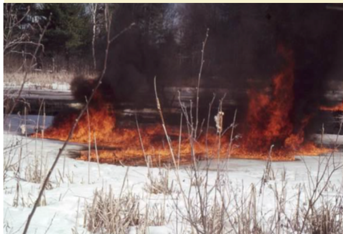
FIGURE 3. ISB conducted in a freshwater marsh in snow. (NOAA 1993)
